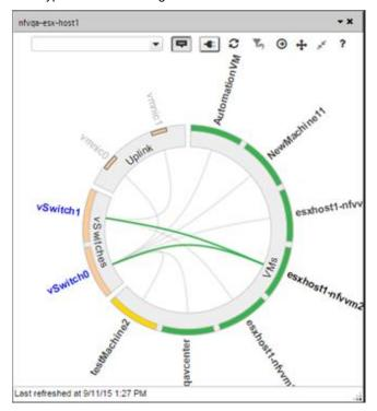
Figure 30: Hypervisor Wheel Diagram Showing virtual switches and L2 Connections
